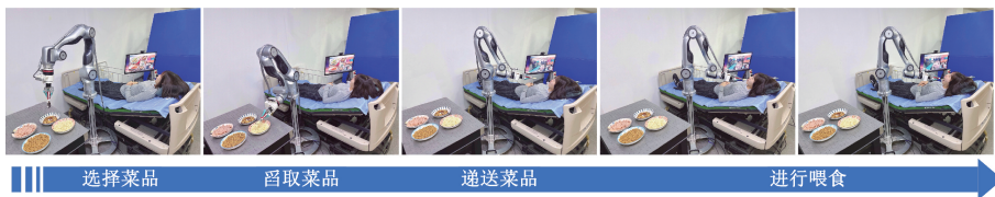
图 17 辅助喂食实验过程 Fig. 17 Experimental process of assisted feeding
